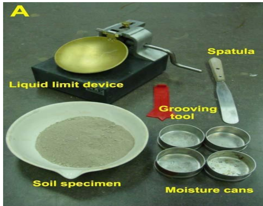
Fig: Shows Liquid limit test apparatus
